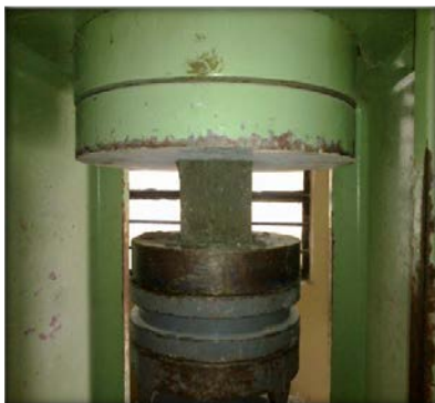
Fig 9 Compression Test on Concrete Cubes(UTM)
