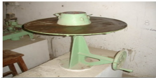
Fig 6 Flow Table Test
