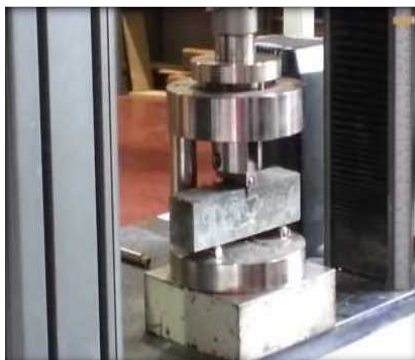
Fig 11 Flexural Strength Test on Concrete Prism
