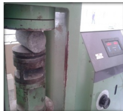
Fig 10 Split tensile Strength Test on Concrete Cylinders(UTM)
