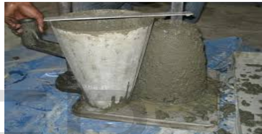
Fig 5 Slump Cone Test
